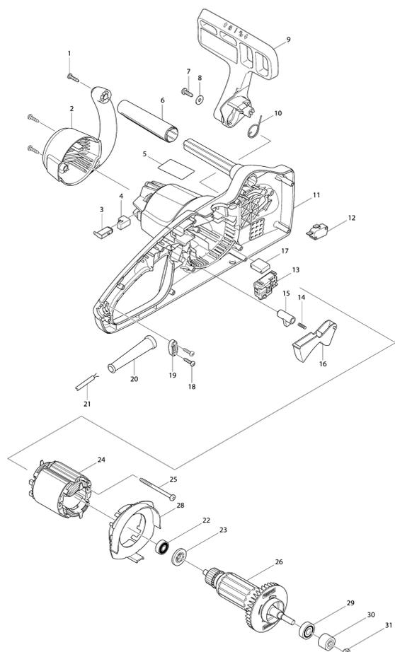
Model No.UC3541A 350MM ELECTRIC CHAIN SAW
