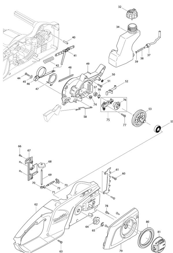
Model No.UC3541A 350MM ELECTRIC CHAIN SAW
