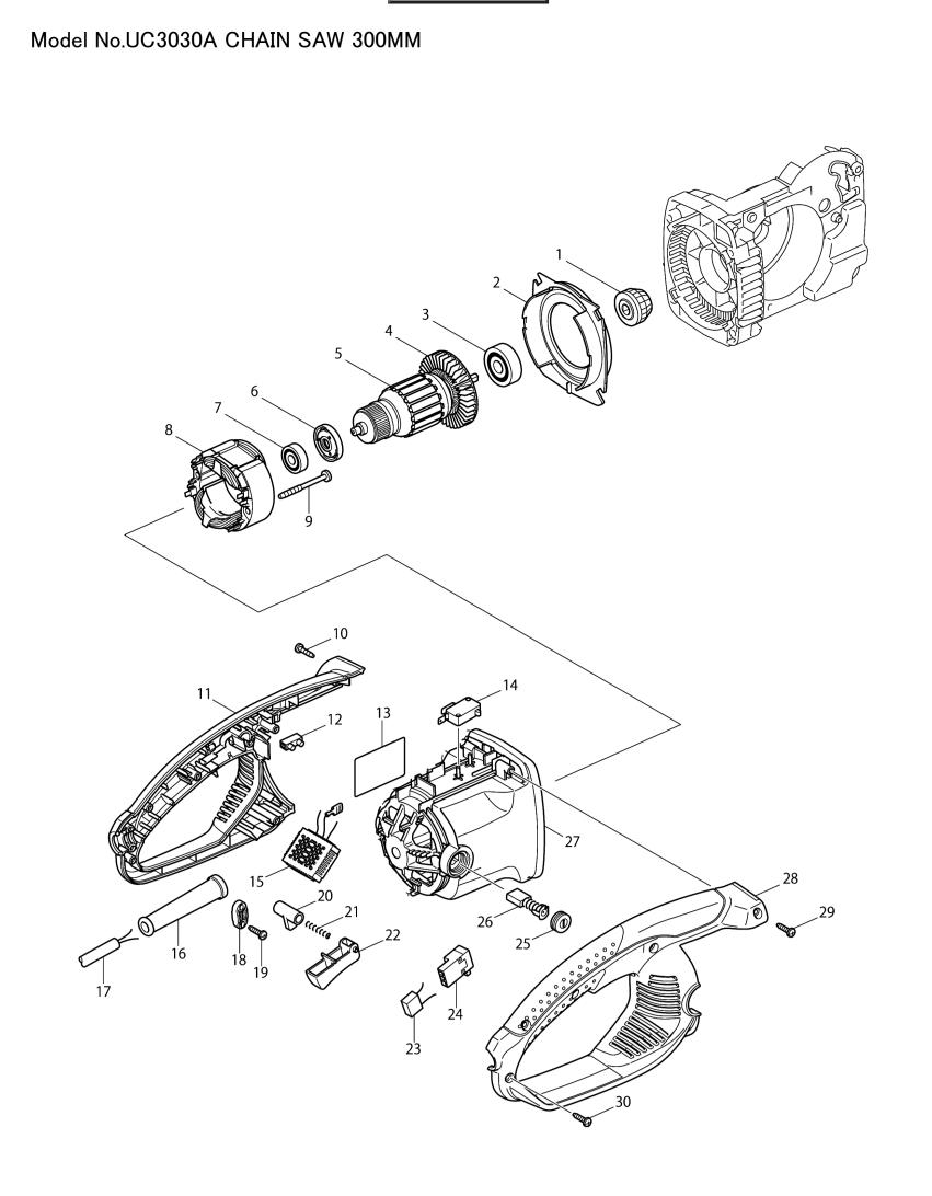
Model No.UC3030A CHAIN SAW 300MM
